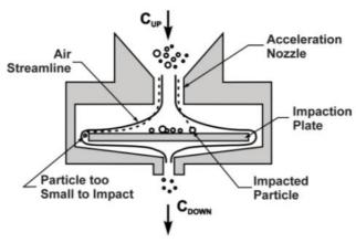
Figure 1. Schematic of an inertial impactor
