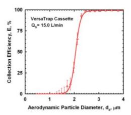
Figure 3. VersaTrap performance at 15L/min
